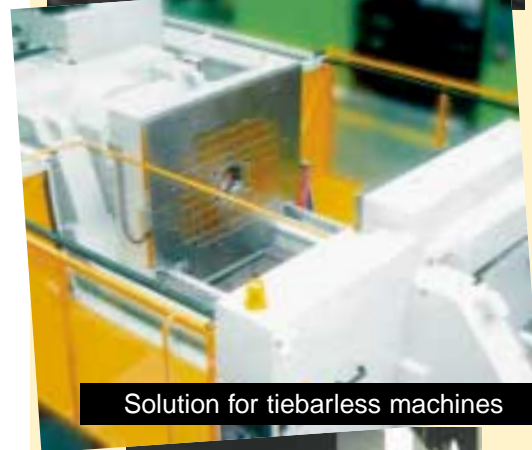
Multi-shot injection with revolving platen.
